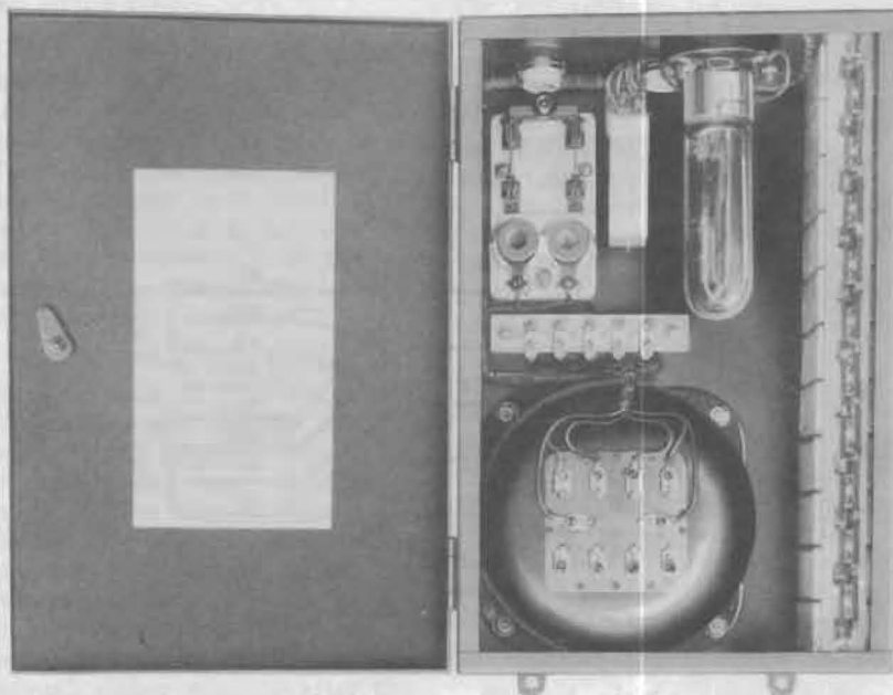
Figure 4—No. 60B Vacuum Tube Rectifier
