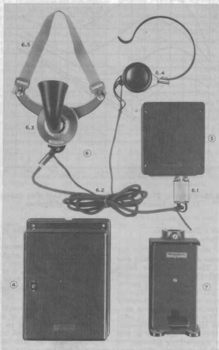
Figure 36—Dispatcher's Station-Telephone Equipment
